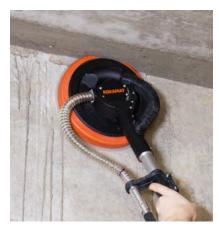
Grinding large surfaces very quickly
